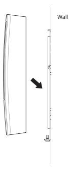
**3** Assemble XPass D2 with the bracket by rotating the product fixing screw.
